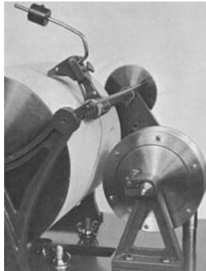
This is one of the earliest mechanical pen and ink strip recorders for measuring tidal levels. Click the image for a larger view.
